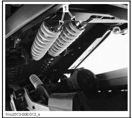
DOUBLE REAR SHOCK 1. Rear springs adjustment
