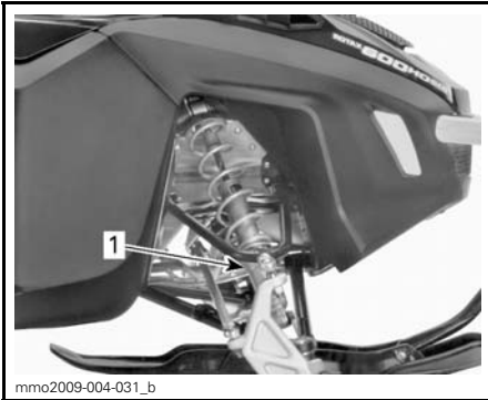
mme2009-004-031_b TYPICAL - CAM TYPE PRELOAD 1. Adjustment cam
