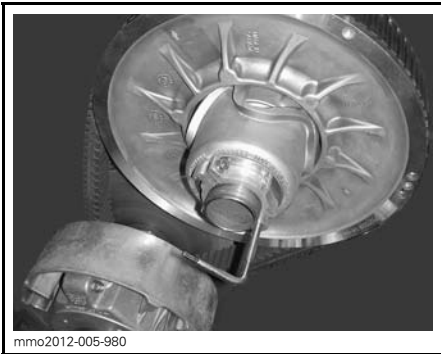
PULLEY EXPANDER INSTALLED ON ADJUSTER HUB
