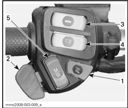
TYPICAL 1. Start/Electronic Reverse button 2. Headlights dimmer switch 3. Heated grips 4. Heated throttle lever 5. Mode/set button
