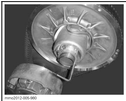
PULLEY EXPANDER INSTALLED ON ADJUSTER HUB
