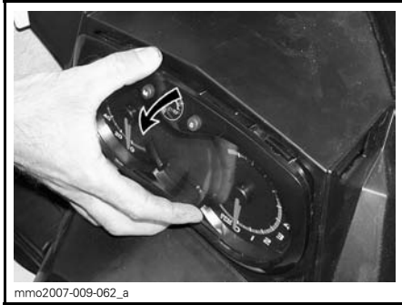
Step 1: Step 1: Push both sides Step 2: Step 2: Pull to release
