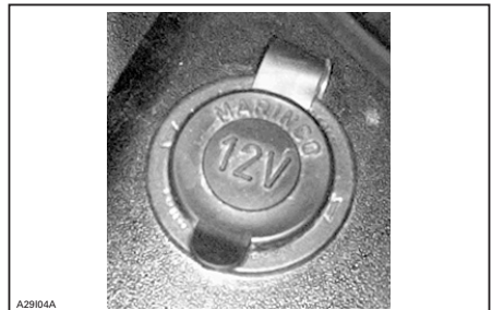
TYPICAL — ELECTRIC POWER OUTLET
