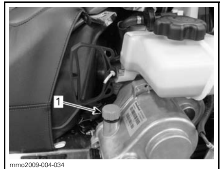
mmo2009-004-034 TYPICAL 1. Filler cap
