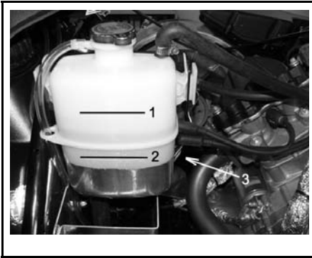
YETI PRO V-800-EXPANSION TANK NEAR THE MUFFLER
