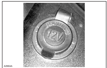
TYPICAL — ELECTRIC POWER OUTLET
