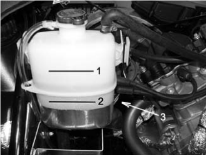
YETI PRO V-800-EXPANSION TANK NEAR THE MUFFLER
