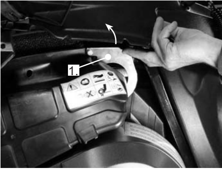
1. Intake silencer clamp.
