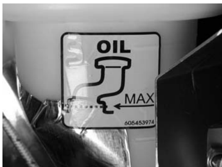
SEE MAX OIL LEVEL DECAL ON THE SIDE OF THE OIL TANK
