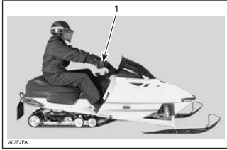
Too hard of adjustment - too much preload 1. Handlebar is very easy to turn – understeering attitude
