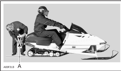
Proper adjustment A. 50 to 75 mm
