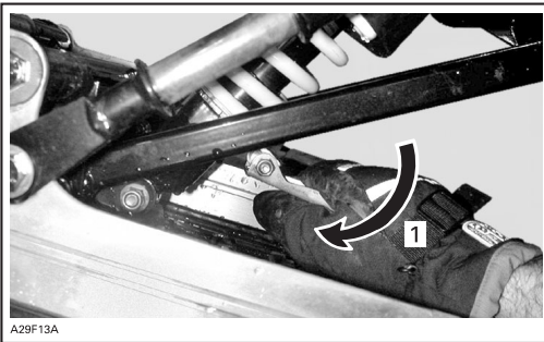
1. From the highest position, turn adjuster to select lowest position then, turn adjuster to the desired position
