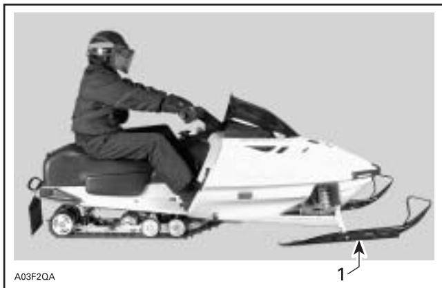
TYPICAL — TOO LONG STRAP 1. Skis lift off the ground
