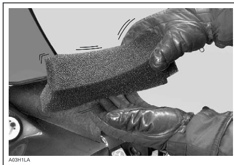
Remove snow from filter on air intake silencer
