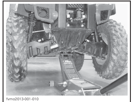
TYPICAL — FRONT LIFTING POINT
