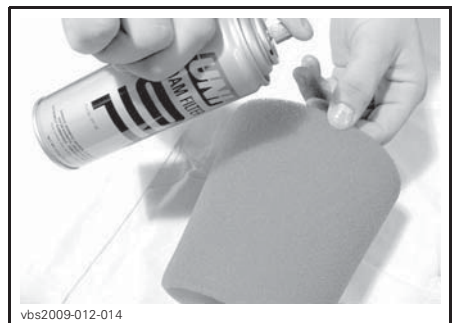
TYPICAL - OIL THE FOAM FILTER
