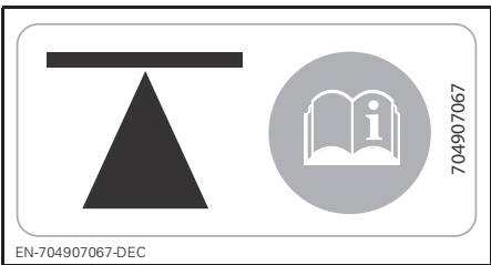
ON SIDE OF CHASSIS - FRONT AND REAR Refer to INSTRUCTIONS FOR VEHICLE LIFTING section in your OPERATOR'S GUIDE for lifting points locations and procedure.
