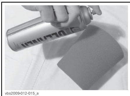
TYPICAL - SPRAY THE FOAM FILTER
