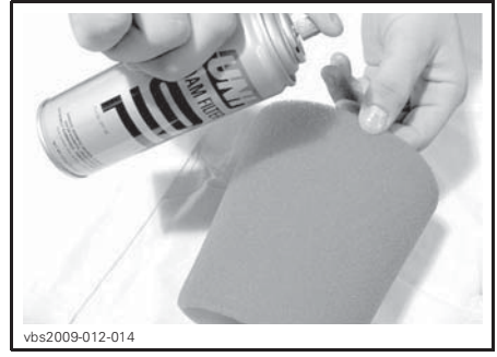
TYPICAL - OIL THE FOAM FILTER
