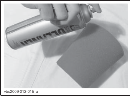
TYPICAL - SPRAY THE FOAM FILTER
