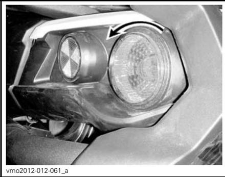
Disconnect the light bulb connector.
