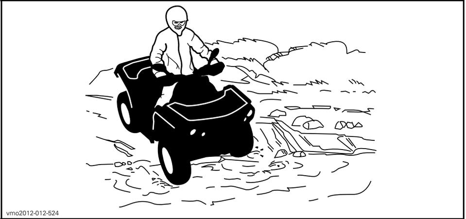
Wet brakes will affect the braking ability of your vehicle. Make sure you dry the brakes by applying them several times after the vehicle leaves the water, mud or snow. Allow greater distance for braking.
