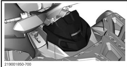
Remove engine coolant reservoir cap.
