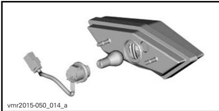
3. Remove bulb socket from taillight. Installation is the reverse of the removal procedure.
