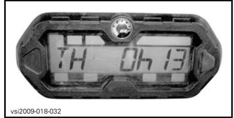
Press and HOLD the selector button for 2 seconds to reset the hour meter.
