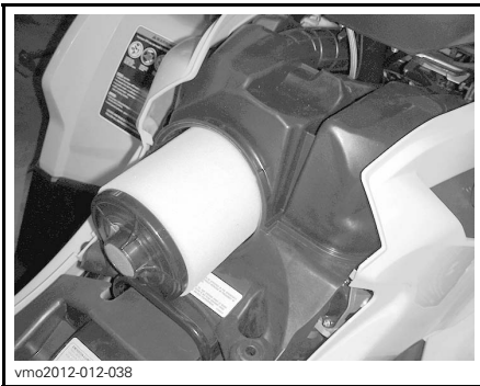
AIR FILTER REMOVAL
