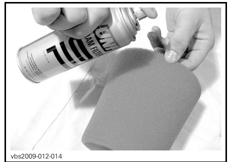
TYPICAL - OIL THE FOAM FILTER
