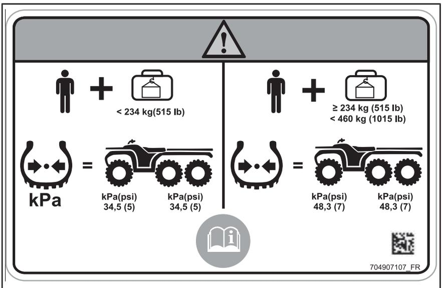
The diagram is enclosed in a rounded rectangle with a warning triangle at the top center. It is divided into two vertical sections by a central line.
