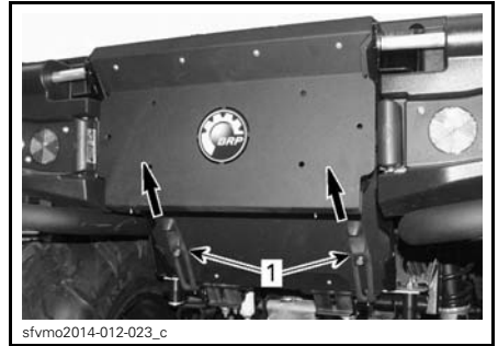
PULL LATCHES UPWARDS 1. Rubber latches
