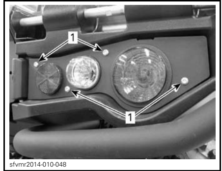
TYPICAL 1. Screws securing taillight assembly
