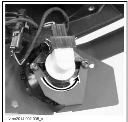
TYPICAL: ROTATE BULB COUNTERCLOCKWISE
