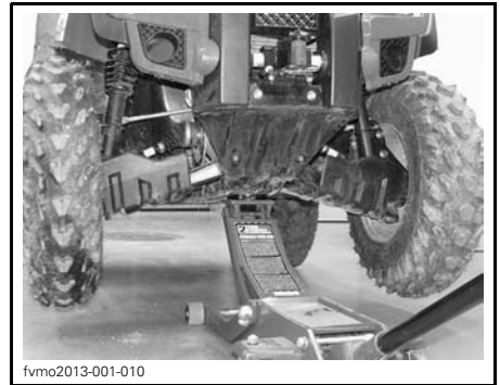
TYPICAL — FRONT LIFTING POINT
