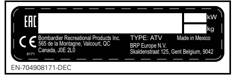
TYPICAL - VIN LABEL - UNDER SEAT
