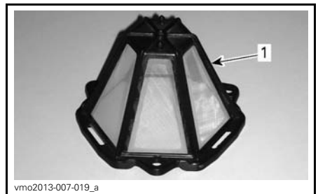
1. CVT air filter (clip-on type)
