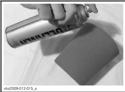
TYPICAL - SPRAY THE FOAM FILTER
