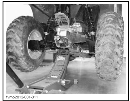
TYPICAL — REAR LIFTING POINT
