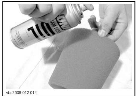
TYPICAL - OIL THE FOAM FILTER
