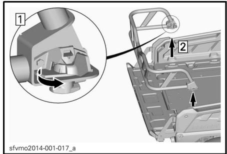
3. Remove support brackets from tail gate.
