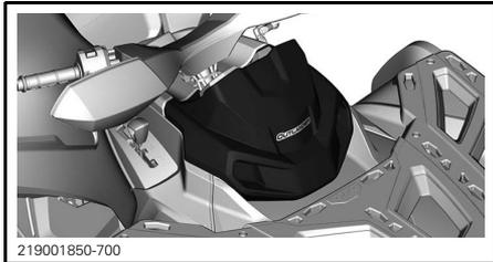
Remove the coolant reservoir cap.
