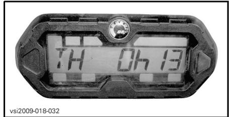
Press and HOLD the selector button for 2 seconds to reset the hour meter.
