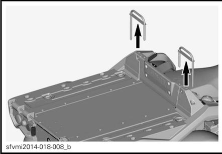
3. Place side wall on flat bed and lower it on its place.
