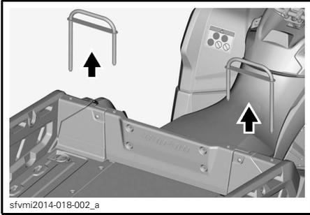
5. Lift side wall up and remove it.
