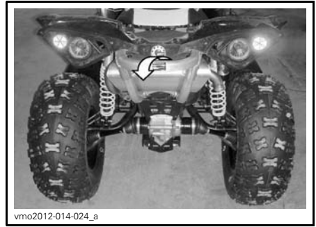
TYPICAL - REAR TIE-DOWN POINT LOCATION
