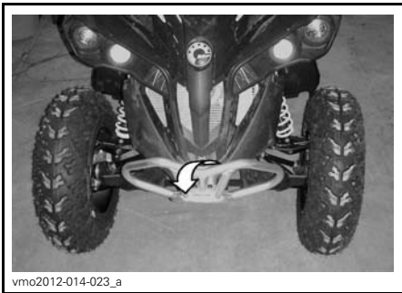
TYPICAL - FRONT TIE-DOWN POINT LOCATION
