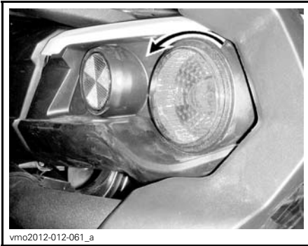
TYPICAL - FRONT TURN SIGNAL LIGHT 1. Retaining screws
