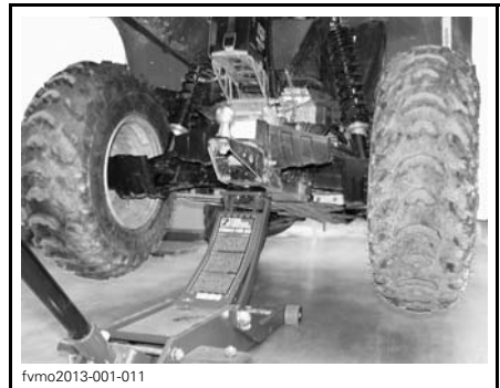
TYPICAL — REAR LIFTING POINT
