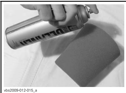
TYPICAL - SPRAY THE FOAM FILTER
