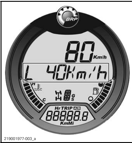
L AND SPEED LIMIT FLASHING
