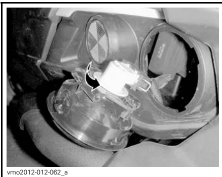
TYPICAL - REAR TURN SIGNAL LIGHT 1. Retaining screws
