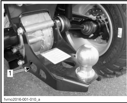
TYPICAL - REAR TIE-DOWN POINT LOCATION
