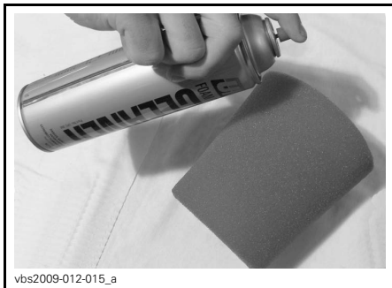
TYPICAL - SPRAY THE FOAM FILTER
