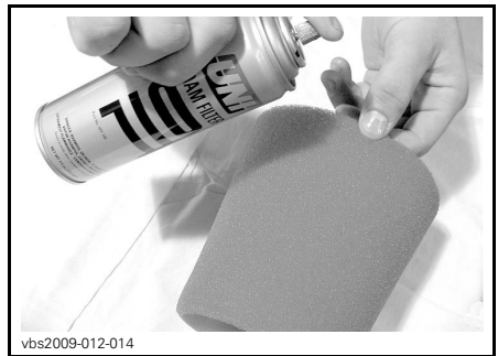
TYPICAL - OIL THE FOAM FILTER
