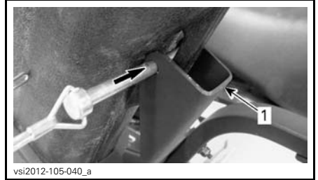
1. Bent plate of gun boot support
