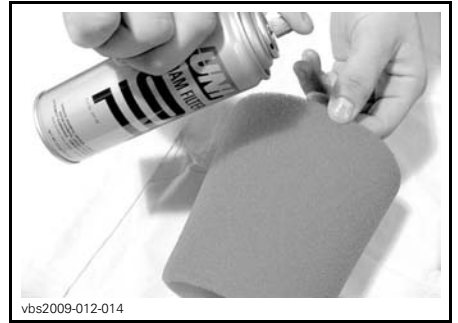
TYPICAL - OIL THE FOAM FILTER
