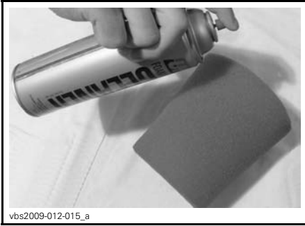
TYPICAL - SPRAY THE FOAM FILTER
