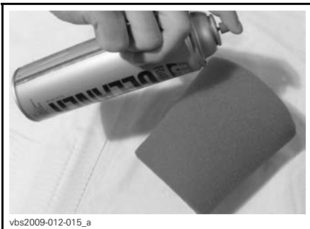
TYPICAL - SPRAY THE FOAM FILTER
