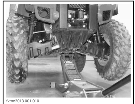
TYPICAL — FRONT LIFTING POINT
