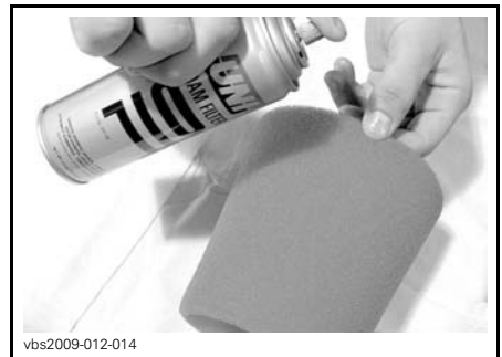
TYPICAL - OIL THE FOAM FILTER
