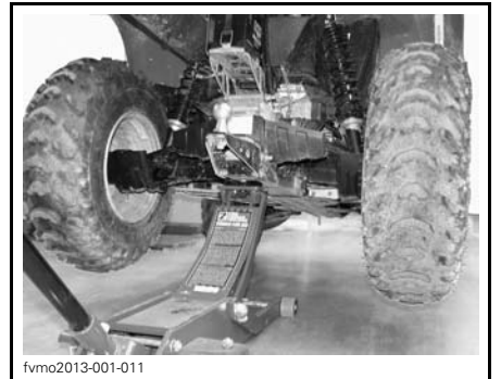
TYPICAL — REAR LIFTING POINT
