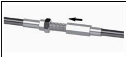
**RETROCEDA A PORCA DE AJUSTE EM UMA VOLTA**
