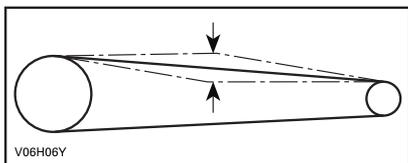
**DÉFLEXION DE LA CHAÎNE D'ENTRAÎNEMENT ENTRE 15 mm and 25 mm**
