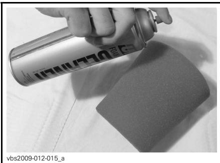
TYPICAL - SPRAY THE FOAM FILTER
