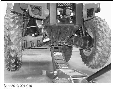
TYPICAL — FRONT LIFTING POINT
