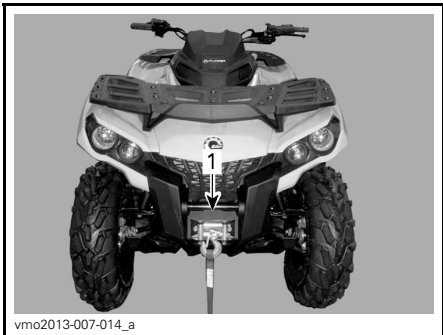
1. Front tie-down point location
