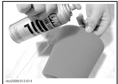
TYPICAL - OIL THE FOAM FILTER
