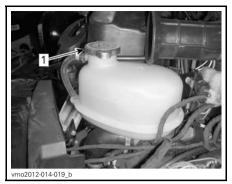
1. Engine coolant reservoir cap
