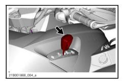
The shift lever is used to change the gearbox position.
