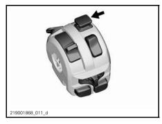
Push the switch down to activate the hazard lights. Pull it up to turn off.
