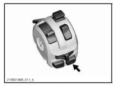
Press and hold the button to start the engine.
