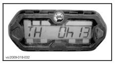
Press and HOLD the selector button for 2 seconds to reset the hour meter.
