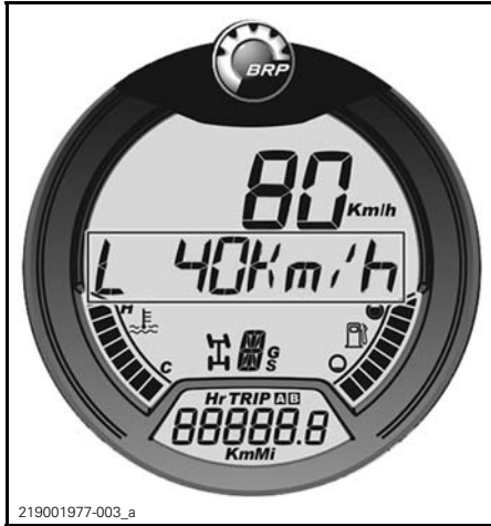
L AND SPEED LIMIT FLASHING
