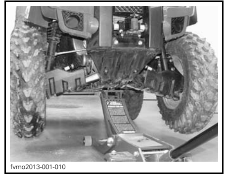
TYPICAL — FRONT LIFTING POINT
