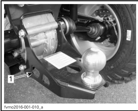
TYPICAL - REAR TIE-DOWN POINT LOCATION
