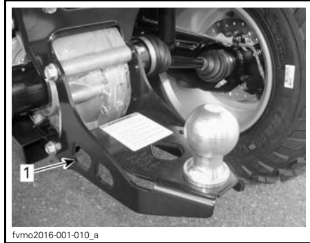
TYPICAL - REAR TIE-DOWN POINT LOCATION
