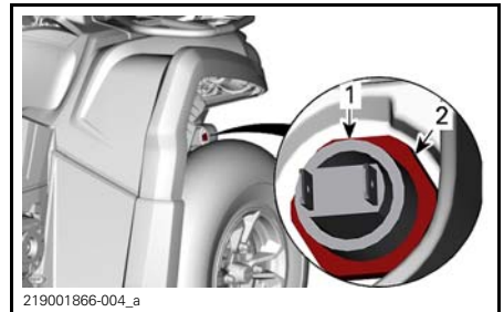
1. Position light 2. Retaining nut
