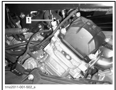
TYPICAL 1. Rear cylinder bleed screw
