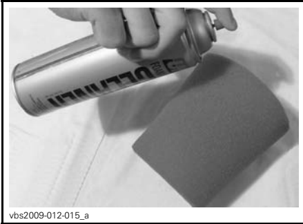
TYPICAL - SPRAY THE FOAM FILTER
