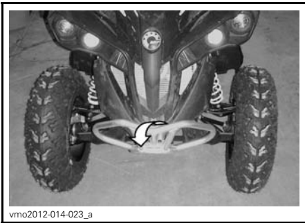
TYPICAL - FRONT TIE-DOWN POINT LOCATION
