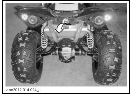
TYPICAL - REAR TIE-DOWN POINT LOCATION
