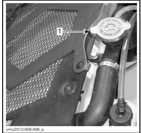
TYPICAL 1. Radiator cap
