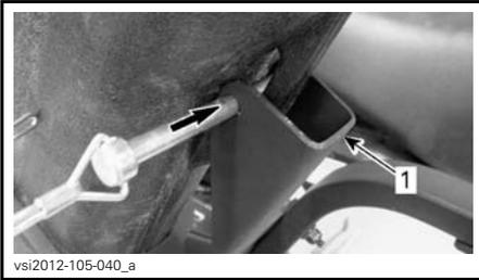
1. Bent plate of gun boot support
