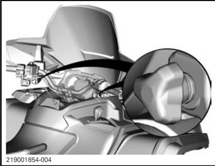
To install, insert the windshield arms into their supports, then hand tighten the knobs.
