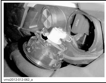
Remove bulb socket from taillight. Installation is the reverse of the removal procedure.
