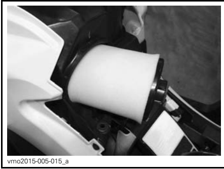
AIR FILTER REMOVAL
