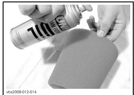
TYPICAL - OIL THE FOAM FILTER
