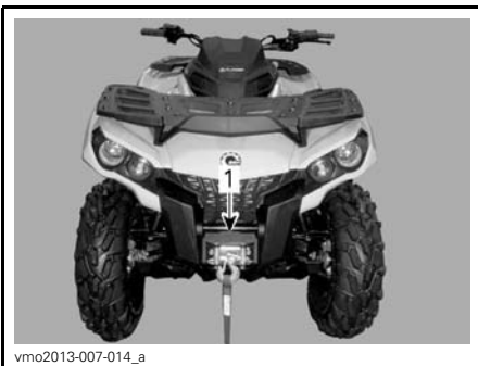
1. Front tie-down point location
