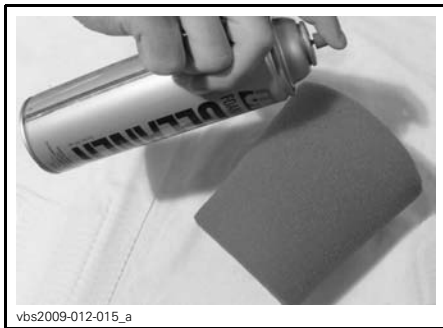
TYPICAL - SPRAY THE FOAM FILTER
