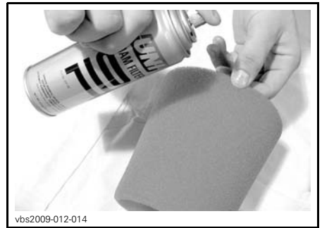
TYPICAL - OIL THE FOAM FILTER
