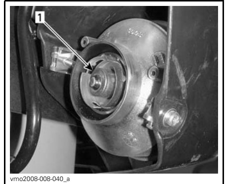
PULL ON BULB TO REMOVE THEN REPLACE BULB 1. Bulb
