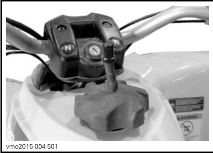
TYPICAL — FUEL TANK CAP
