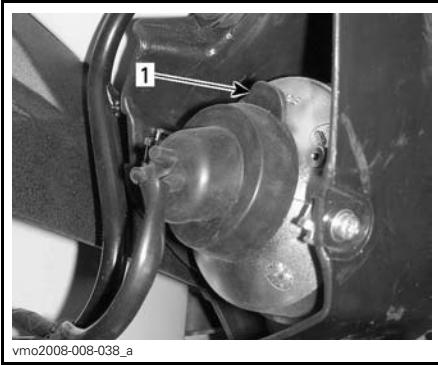
REMOVE RUBBER PROTECTOR 1. Rubber protector
