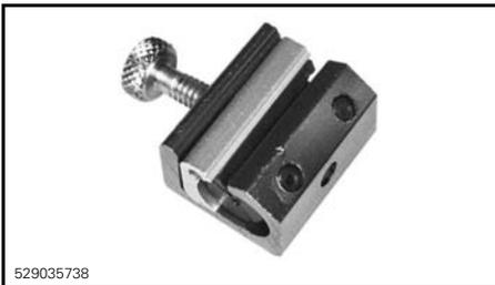
Insert the needle of spray can in the cable luber hole.
