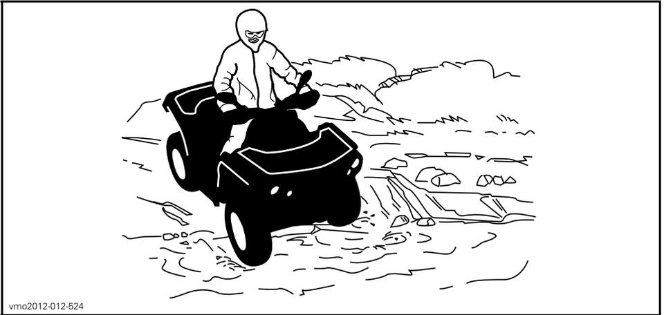
Wet brakes will affect the braking ability of your vehicle. Make sure you dry the brakes by applying them several times after the vehicle leaves the water, mud or snow.
