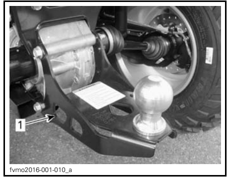
TYPICAL - REAR TIE-DOWN POINT LOCATION
