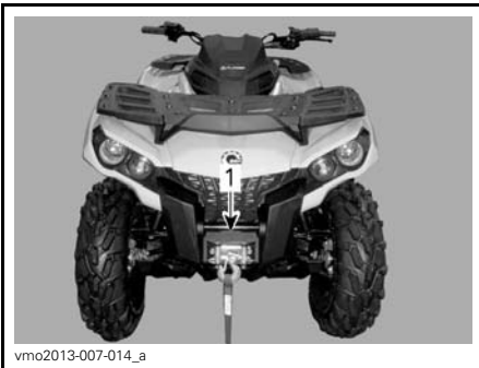
1. Front tie-down point location
