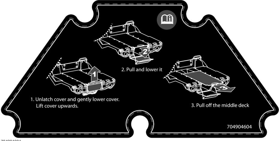
1. Unlatch cover and gently lower cover. Lift cover upwards.
