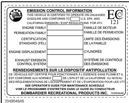
APPLICABLE WHEN EQUIVALENT TO A MODEL CERTIFIED TO US EPA STANDARDS LOCATION: UNDER SEAT, ON THE UPPER FRAME MEMBER
