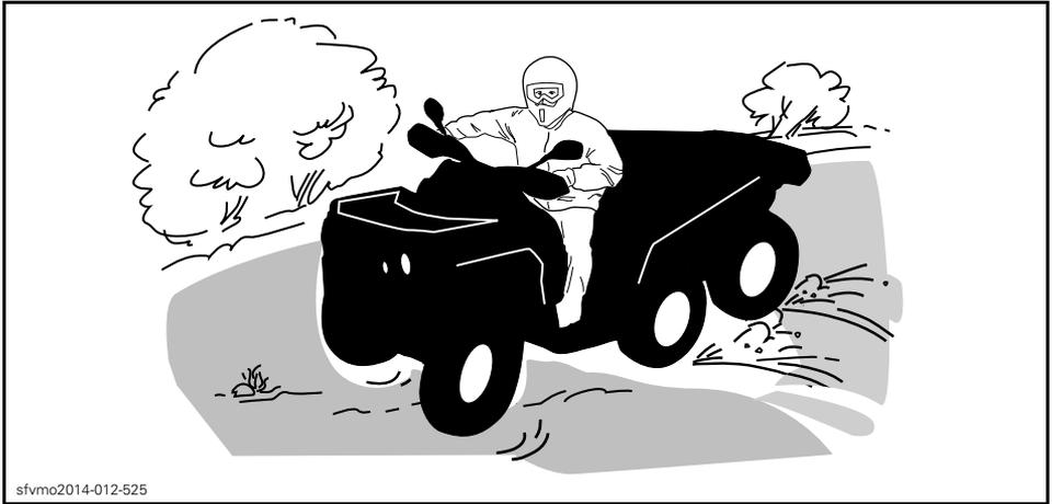
If you do get into a slide or skid, it may help to turn the handlebar in the direction of the skid until you regain control. Never jam the brakes and lock the wheels.
