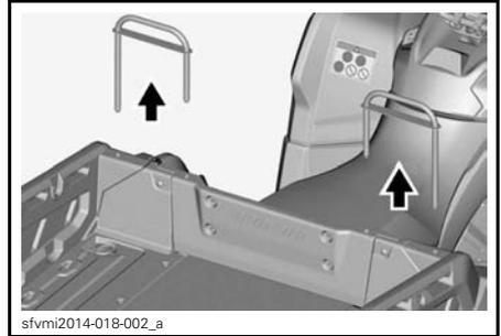
5. Lift side wall up and remove it. Repeat on other side.
