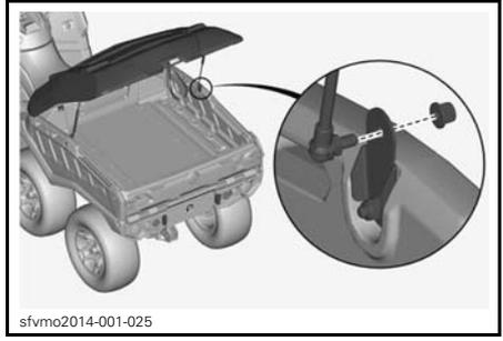
9. Install the shock's top end by screwing it into place.
