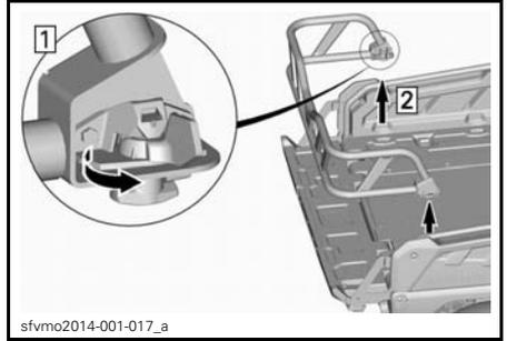
3. Remove support brackets from tail gate.
