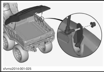
3. Remove pins from hinges both sides.
