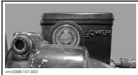
LH REAR BRAKE FLUID RESERVOIR
