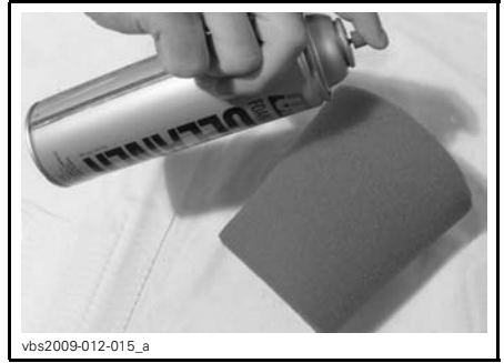
TYPICAL - SPRAY THE FOAM ELEMENT
