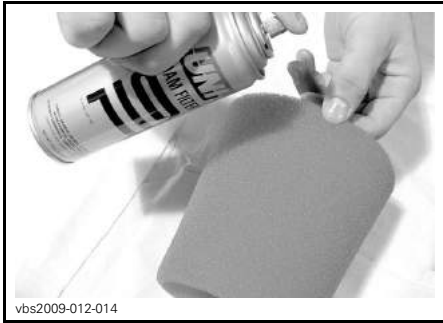
TYPICAL - OIL THE FOAM FILTER
