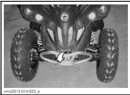
TYPICAL - FRONT TIE-DOWN POINT LOCATION
