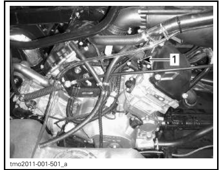
1. Front cylinder bleed screw
