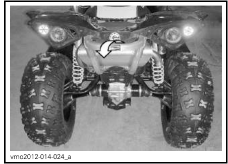
TYPICAL - REAR TIE-DOWN POINT LOCATION
