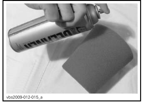
TYPICAL - SPRAY THE FOAM FILTER
