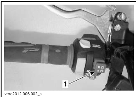
1. Emergency engine stop switch
